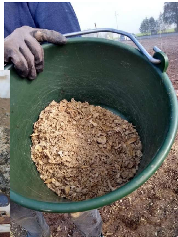
Air-dried and sieved sediments for field application
