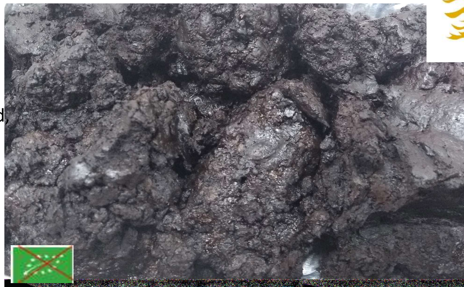
Residual material = «algae fibre»; ca. 15 tons/week, currently incinerated
