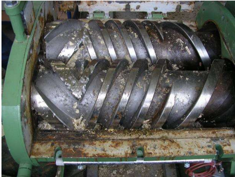
Figure 1. Twin-screw extruder for fibre production at ATB opened to show the mechanism
