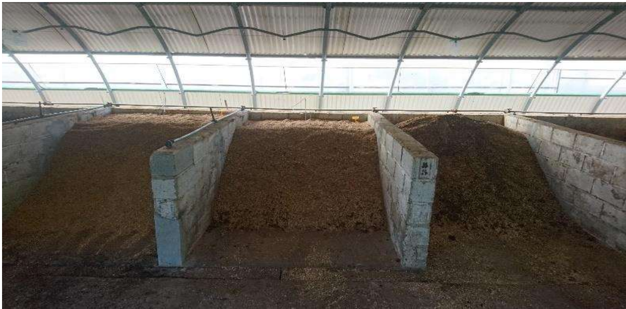
Figure 10. Six m 3 composting piles based on Mediterranean forest biomass and horse manure (pilot composting plant in Cabrils)
