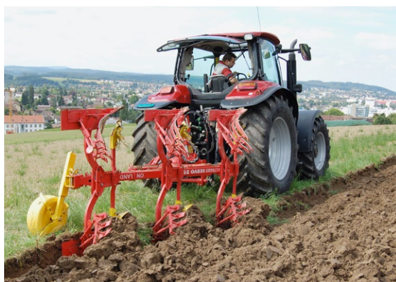
The on-land plough prevents soil compaction in the plough pan.
