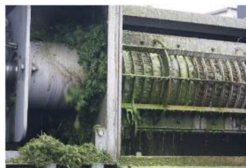
Figure 2: Screw pressing of fresh clover grass into green juice and press cake. Photo: Erik Fog, SEGES
