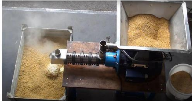
Photo 2: Extrusion technology uses a combination of pressure and friction to generate processing temperature. Photo: www.farmet.cz/en
