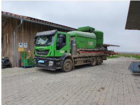
Figure 5: Mobile grinding and mixing plant. Photo: Christopher Lindner
