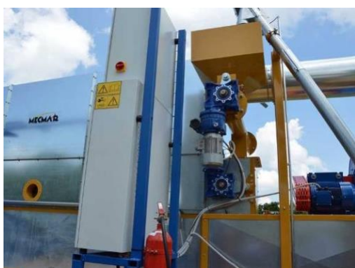
Grain receiving area on mobile soy roaster.
