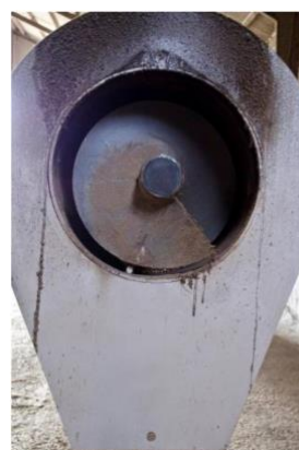
Exit point for the roasted soybeans.
