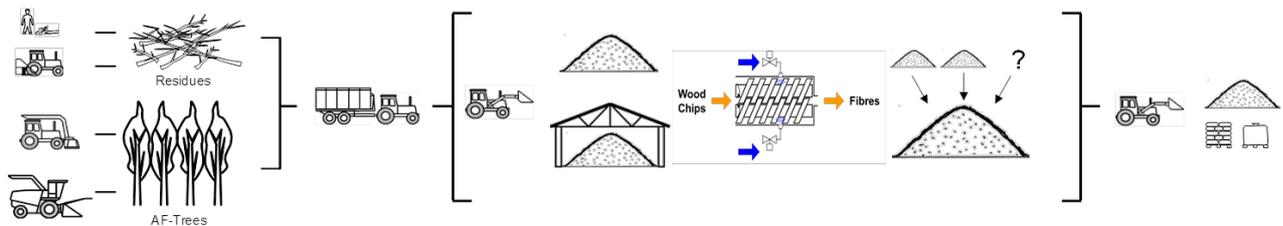
Figure 1 Process chain of lignocellulosic materials from agriculture/forest residues to fibres.
