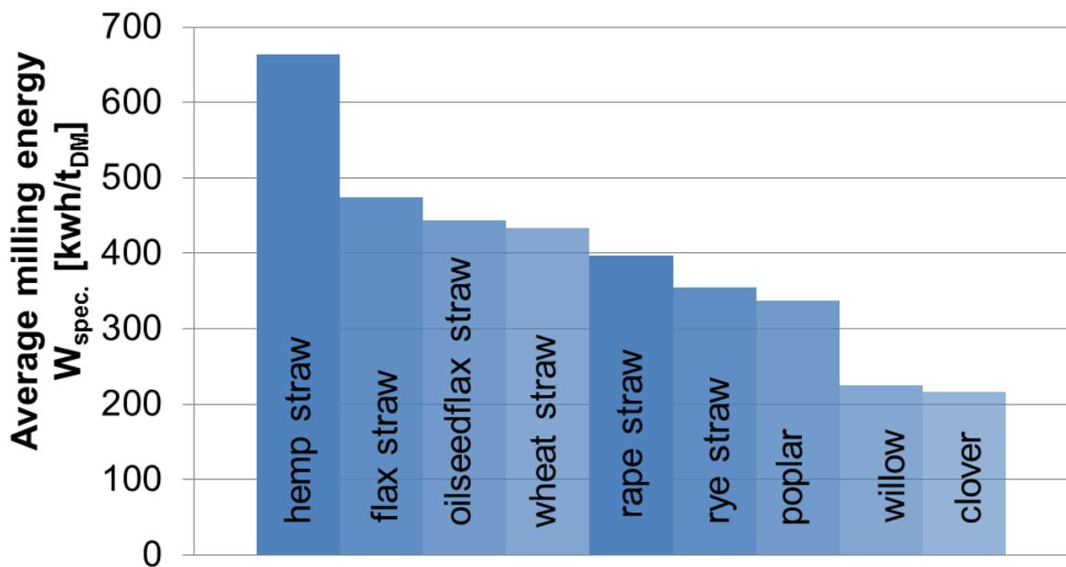
Figure 7 Average milling energy consumed by the extruder in kWh/t<sub>DM</sub> at moisture content of approx. 40 % for various types of input material (Source: ATB)
