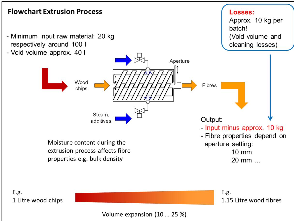
Figure 6. Flowchart showing inputs and outputs of the extrusion process at the ATB pilot plant.
