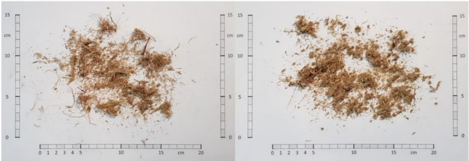
Figure 5 Vine prunings after extrusion and blow drying. Left side (coarser end product) was extruded at 50 % moisture content right side (finer end product) at 40 %. (Source: ATB)
