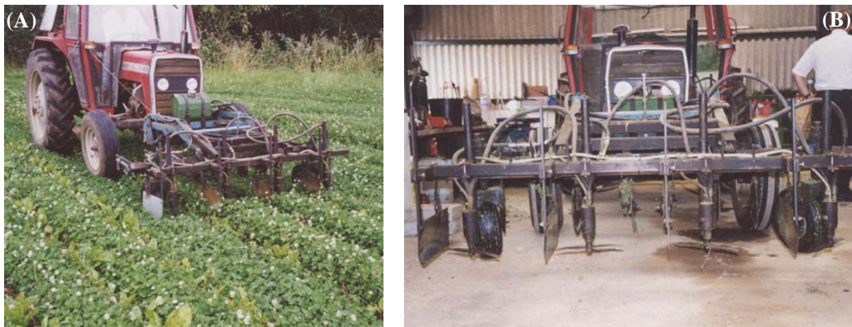
Plate 8. (A) The strip mower used to manage the white clover. (B) Side guards control the lateral movement of clover mulch.
