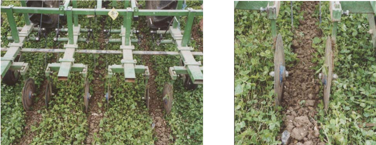
Plate 7. The cultivator (with disc cutter attached) used to manage the clover/crop interface.
