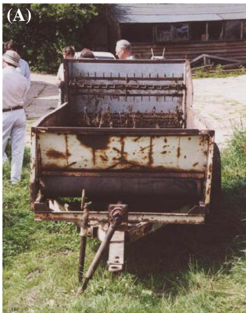
Plate 9. (A) Modified muck spreader for compost applications, and (B) Simple trailed irrigator.
