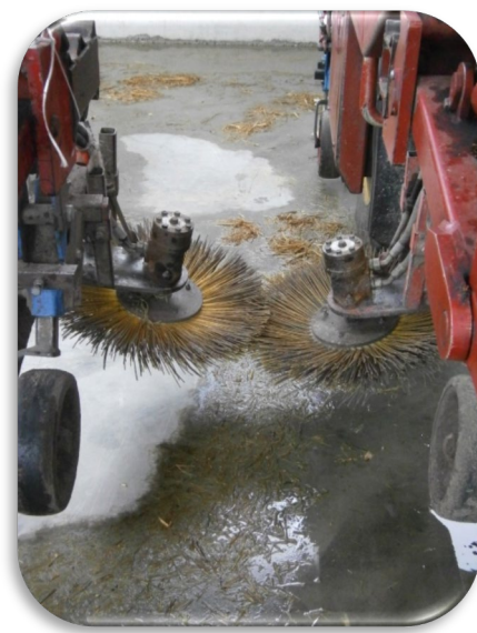
Picture 4: Double brush on high wheel tractor. Photo: Bertels Baumschulen.
