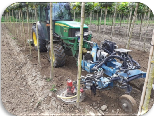
Picture 1: Weed control with movable brush arm in front hydraulics. Photo: Bertels Baumschulen.
