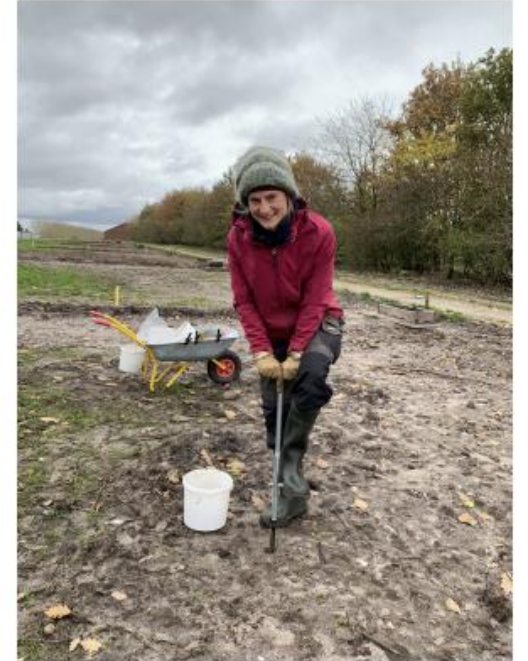
Figure 7.6 Soil sampling with an auger on 31 October 2023. Photo: Kristine Vigh Riis.
