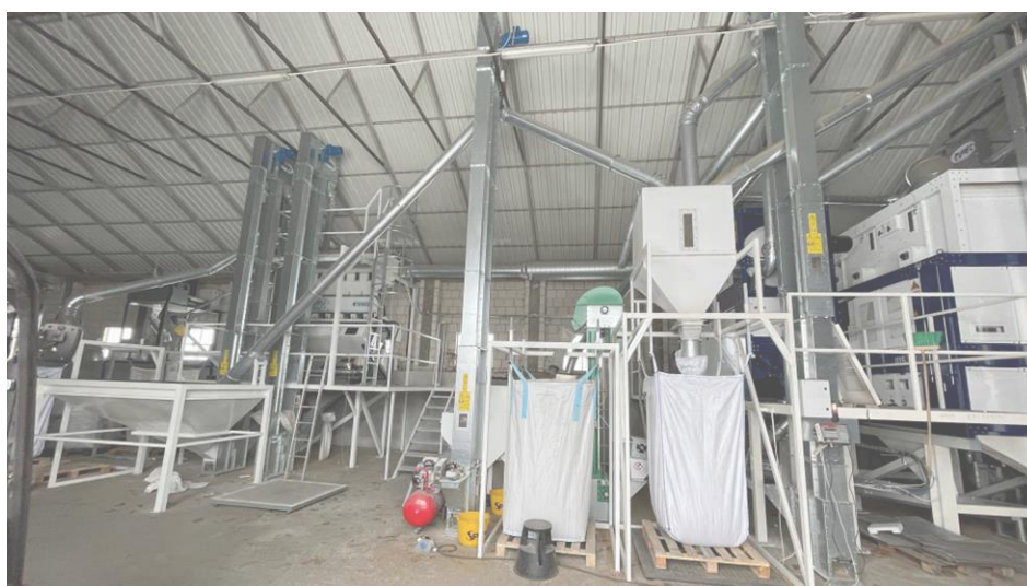
Fig. 2. Cleaning and separation line used in SCOOP project for cleaning and separation of camelina and companion crop seeds
