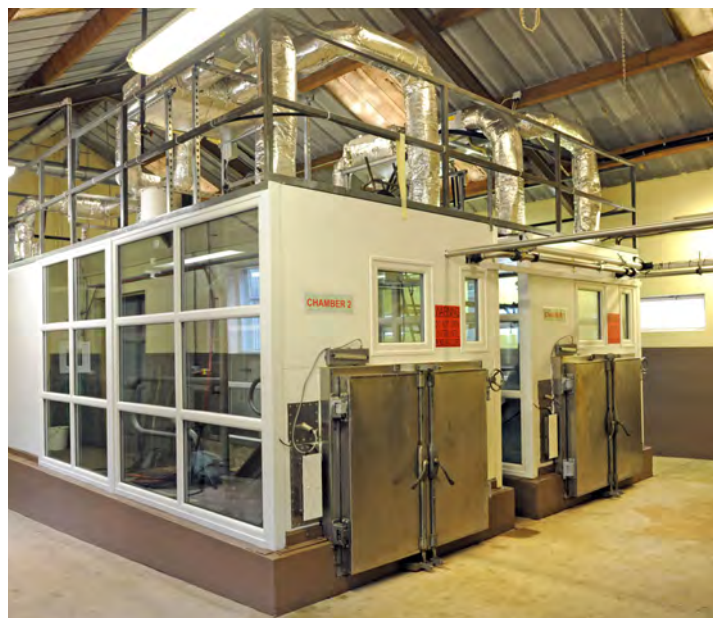
Respiration calorimeter at AFBI-Hillsborough in Northern Ireland – used to measure energy utilisation in cattle
