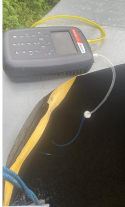
Bilde 13. Biogas5000 Gas Analyser (Geotech: https://cadmus.co.uk/geotech-bioqas-5000-portable-analyser ). Foto: NORSØK
