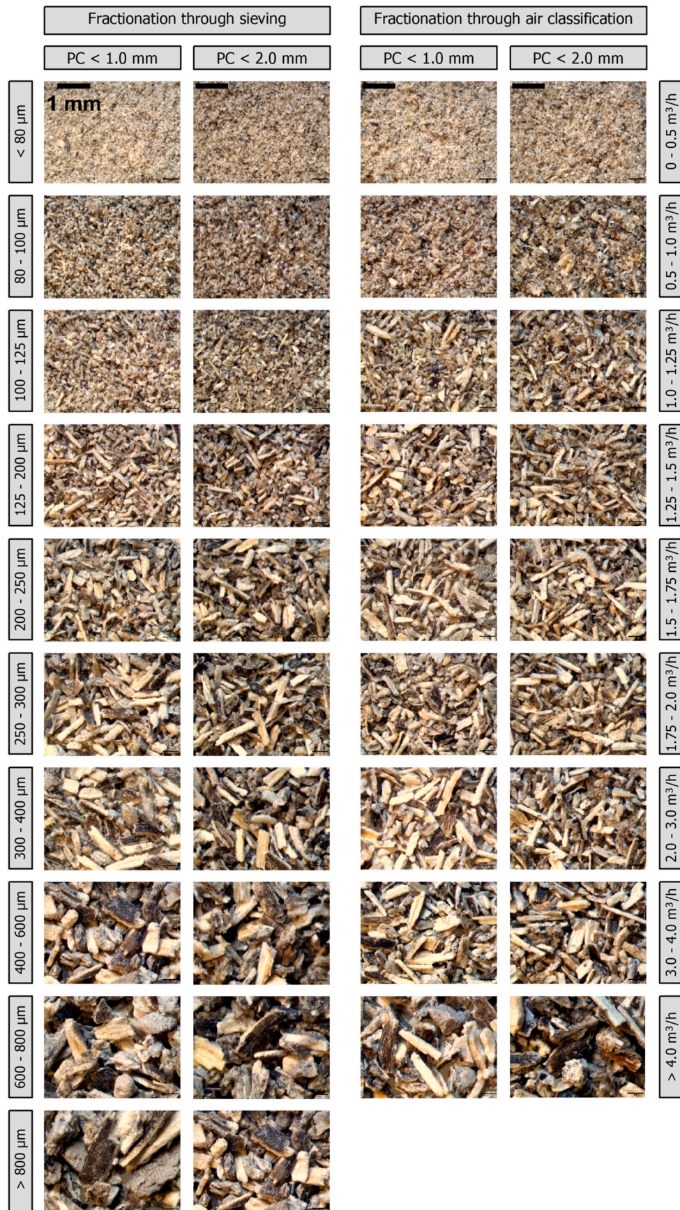
Fig. 3. Microscopic images of individual fractions of deoiled sunflower press cake (PC) milled to < 1.0 mm or < 2.0 mm obtained by sieving or air classification. Scale bar (1 mm, top row) is identical for all images.
