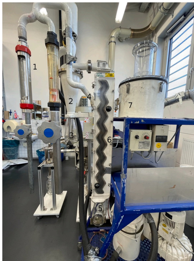
Fig. 1. View of the ziczac air classifier. 1, adjustment of air volume flow; 2, cyclone; 3, fines fraction collection unit; 4, air inlet; 5, coarses fraction collection unit; 6, ziczac channel; 7, vibratory tubular feeder.
