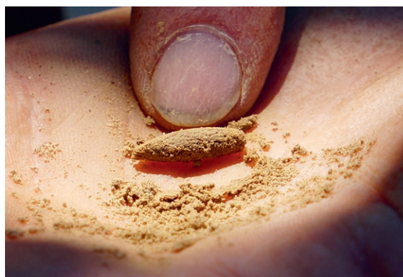
The longer the ribbon can be rolled before it breaks, the higher the clay content of the soil. The sample on the photo is from a sandy soil with little clay content.
