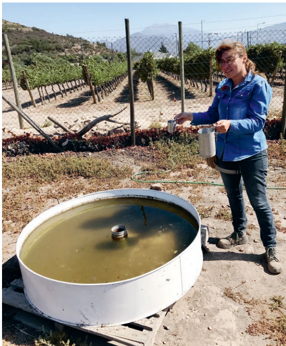
Evaporation pan (left) and weather station (right), as used for measuring reference evapotranspiration ET o .
