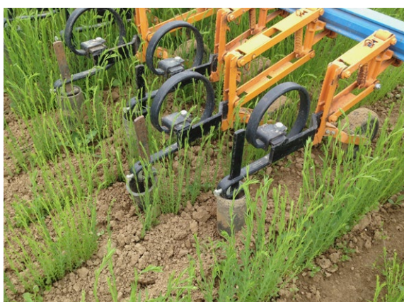
From a row spacing of 20 cm, the crop can be hoed with or without automatic guidance technology.
