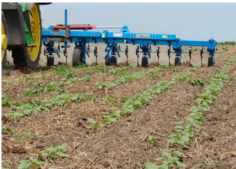
With a row spacing between 50 and 75 cm, sunflowers can be hoed fairly easily with common arable weeding equipment.
