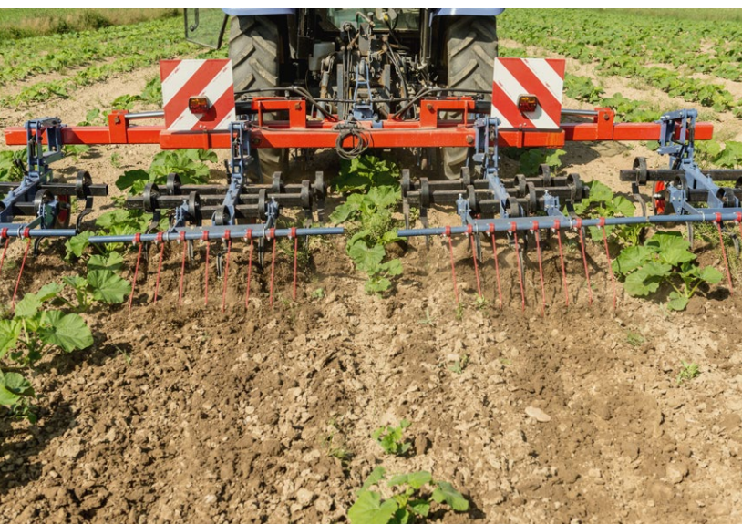
Instead of a harrow, an adapted tine harrow with gaps in the range of the plant rows can be used.
