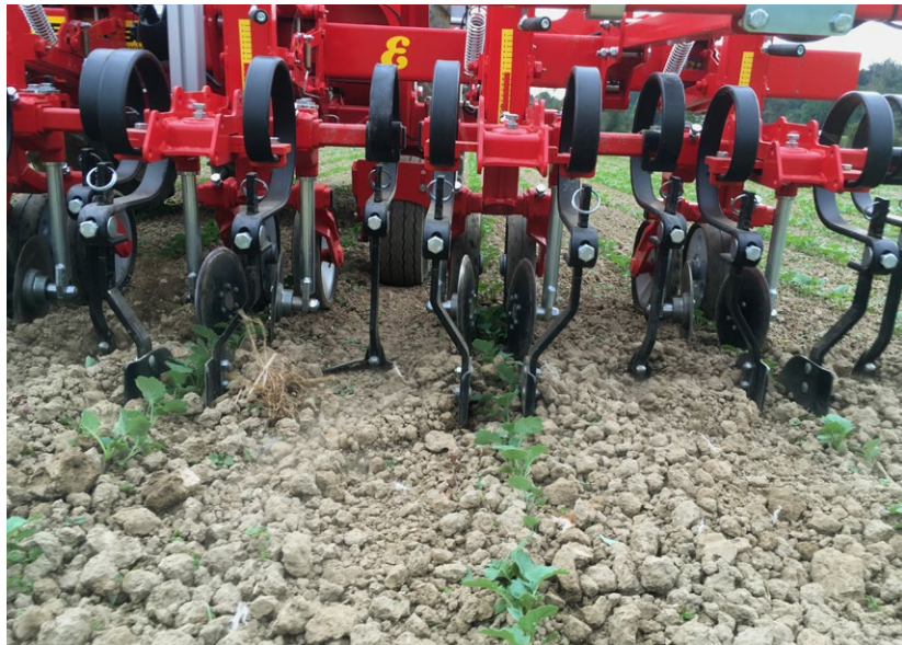
From the 4-leaf stage until the beginning of bolting, rape can be hoed with the duckfoot-tine hoe. Its blades not only control small weeds, but also larger weeds up to the 8-leaf stage. In addition, the blades loosen superficial soil encrustation and stimulate the mineralisation of nitrogen in the soil.
