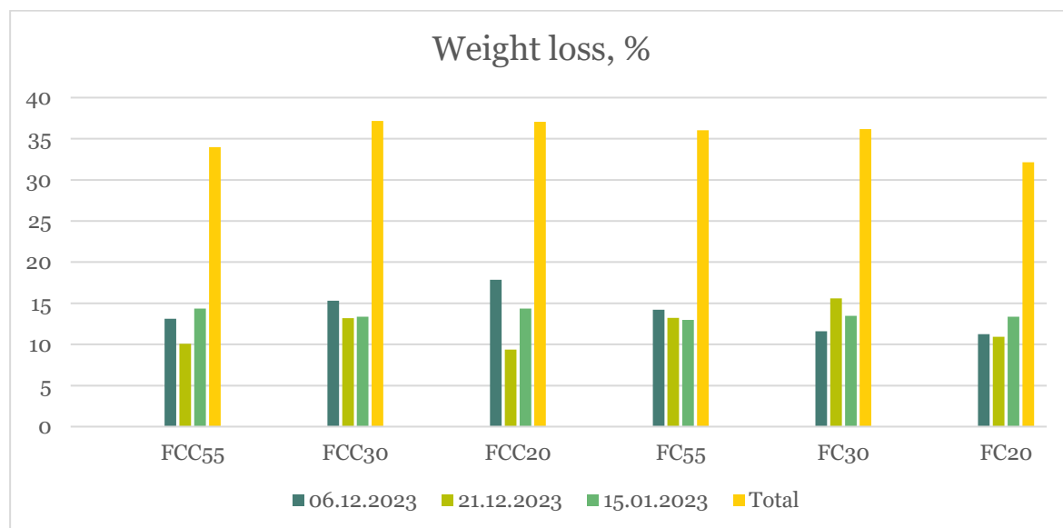
Figure 4. Weight loss (average values per treatment) in Dewar flasks over time, measured between dates when flasks were filled and emptied (and filled again). Treatments = filter cake with and without coagulant (FC, FCC) with various C/N ratios after amendment with fish meal.
