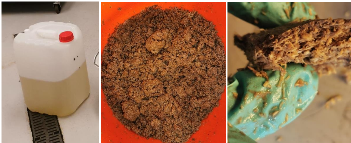
Picture 1 From left: Sludge from a RAS tank with rainbow trout (body size ca. 150 g) fed by certified organic fish feed, compiled in a sludge cone, ready for production of filter cake. Middle: Filter cake from woody material (lignocellulose). Right side: Detail of filter cake. Photos: Carlos Letelier-Gordo.
