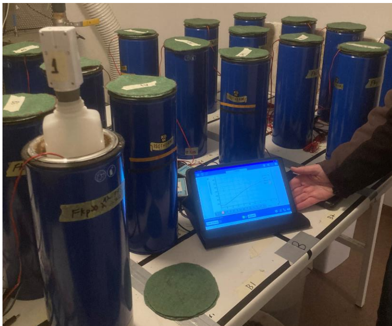
Picture 2 Dewar test flasks for measurement of self-heating in fibre cake material from lignocellulose and fish sludge, with measurement of respiration in the bottle in the bottom left corner. The tablet shows the emission curve (respiration). Photo by AK Løes, December 6, 2023.
