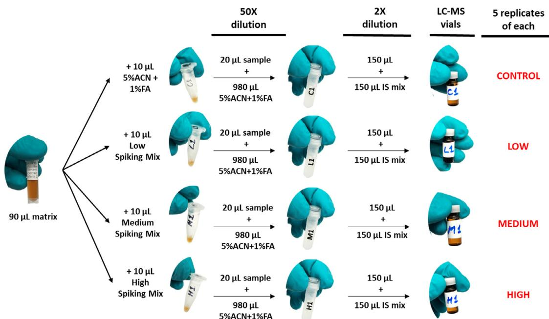
**Fig. 2.** Sample preparation steps for spiking experiment. Bark extract was spiked with using three levels of concentration (final concentration in sample: 10 ng/mL for low level; 20 ng/mL for medium level; 100 ng/mL for high level). The concentrations were calculated based on the stock 1 solution of standards accordingly to the dilutions and necessary spiking level. Spiked samples were prepared as regular samples following a dilution of 100-fold before LC-MS analysis.
