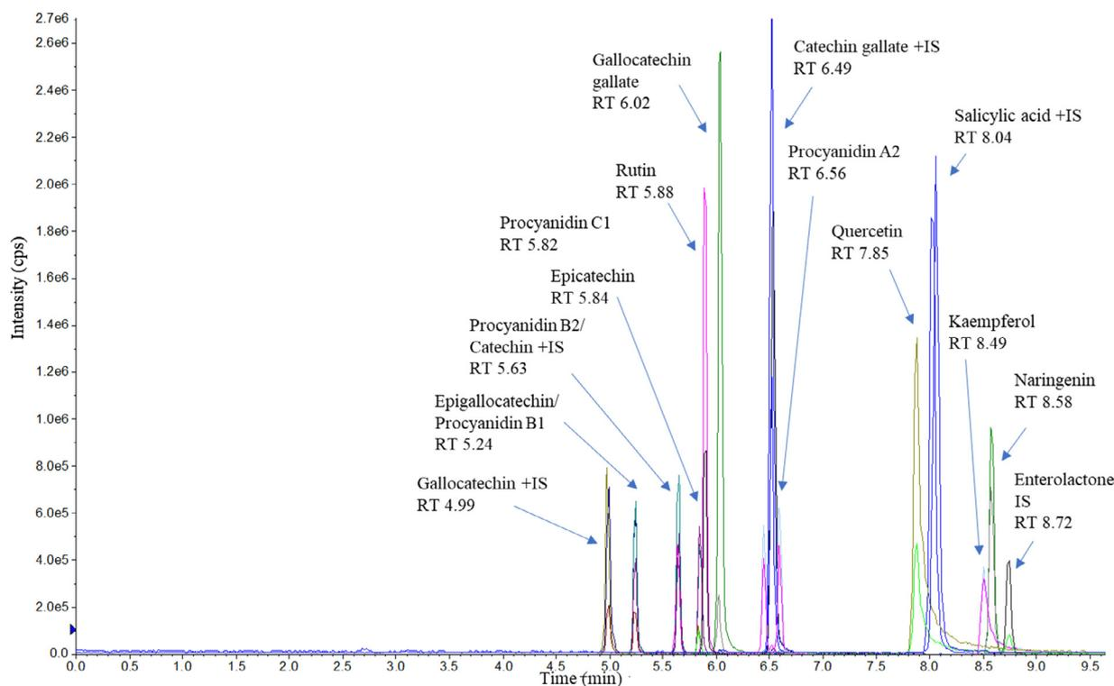
**Fig. 3.** MRM chromatogram of all standards and internal standards (IS) with the corresponding retention times (RT).
