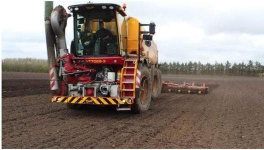
Farm-scale Machine for injection after ploughing/harrowing
