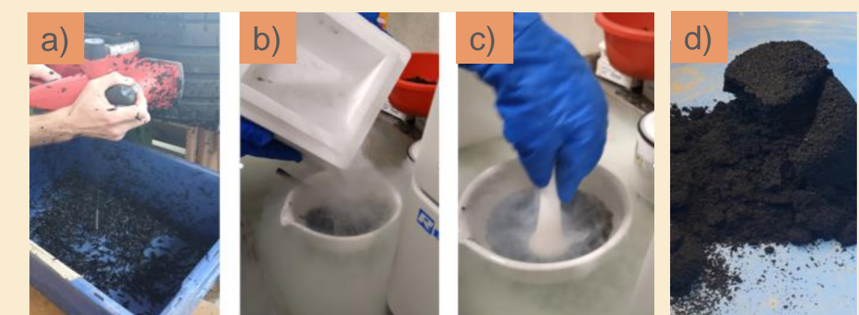
Fig. 1. TP production. a) generation of tyre curls, b) and c) freeze d) final TP.
