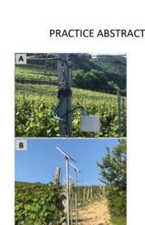
Figure 2: A) Device transmitting VS along the vibrational control grapevine leafhopper; B) the vibrational device and Bioger® (Italy).
