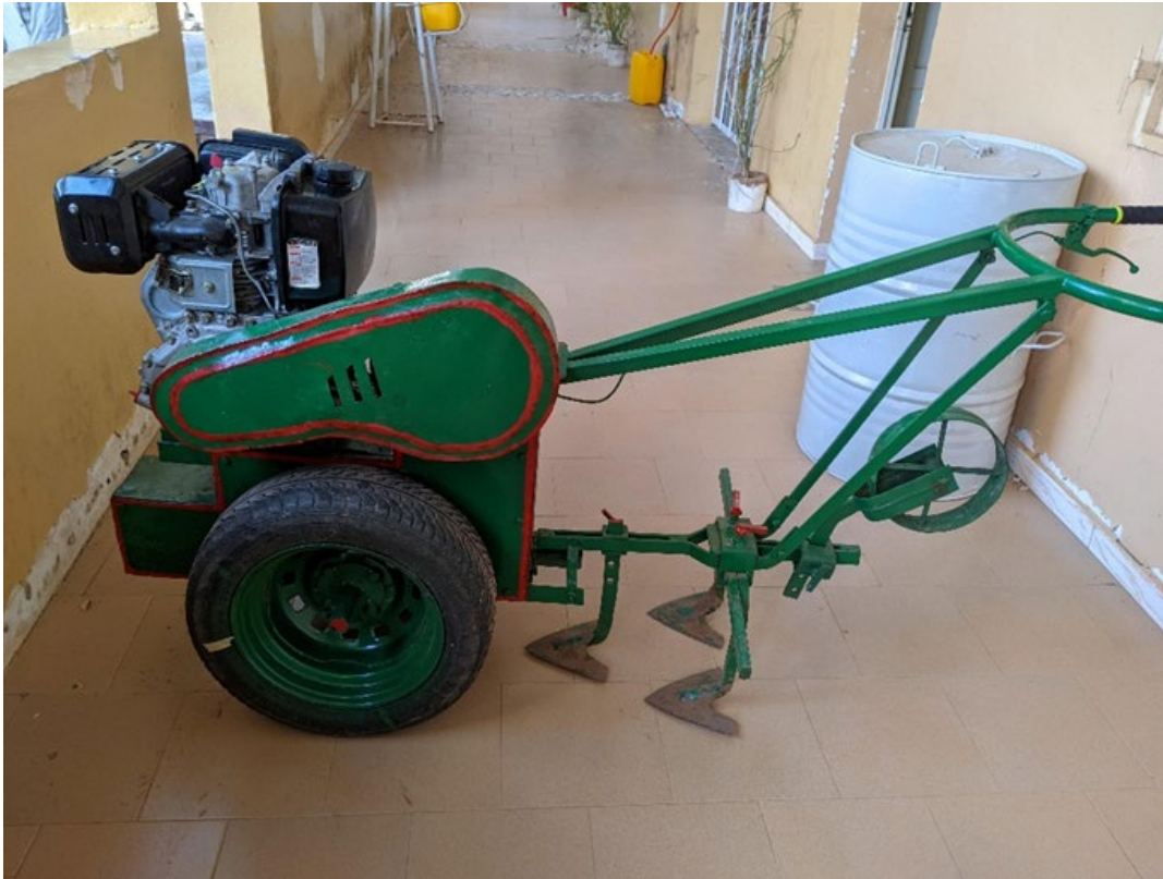
A two-wheeled tractor with weeding sweeps from Senegal.
