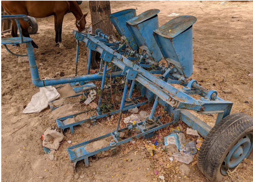
A 4 row planter modified for tractor use from Senegal.
