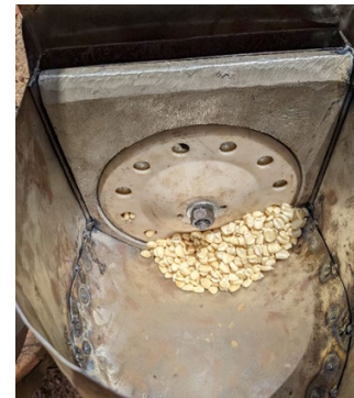
A direct injection planter with fertiliser hopper from South Africa without coulter for planting into mulch.
