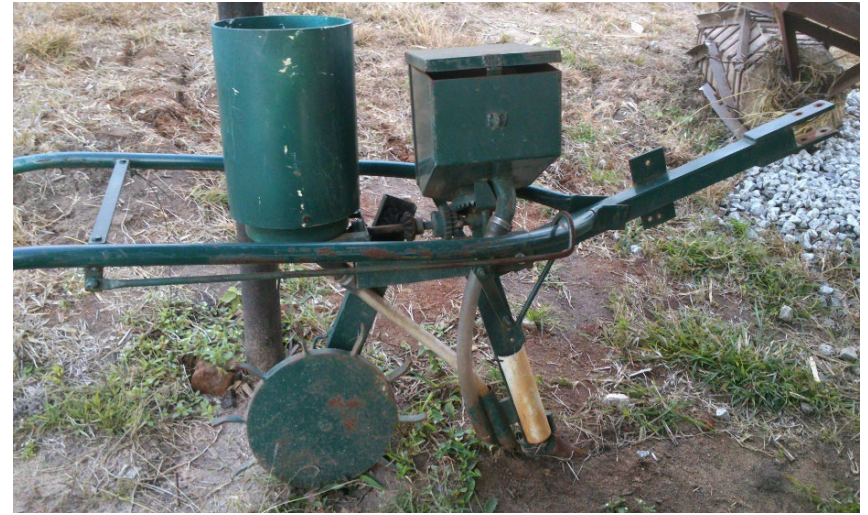
A direct injection planter with fertiliser hopper from South Africa without coulter for planting into mulch.
