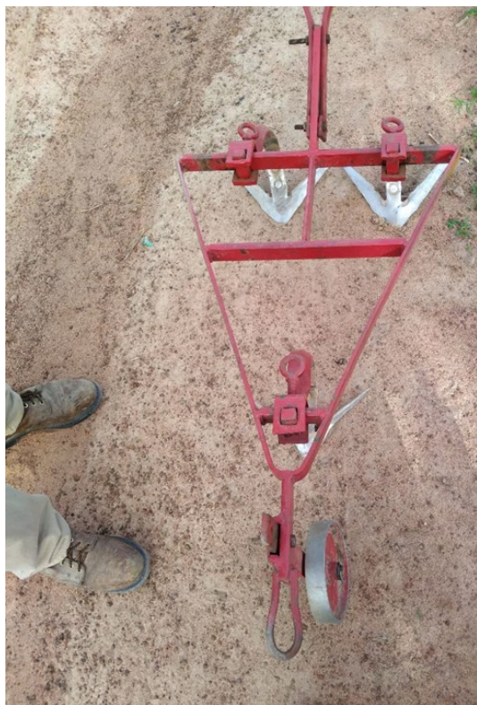
Weeder from Burkina Faso with three sweeps with low angle low crown for shallow weeding
