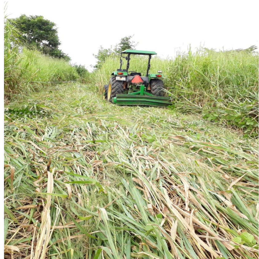
A tractor-drawn roller crimper used by the Centre for No Till Agriculture at Amanche in Ghana
