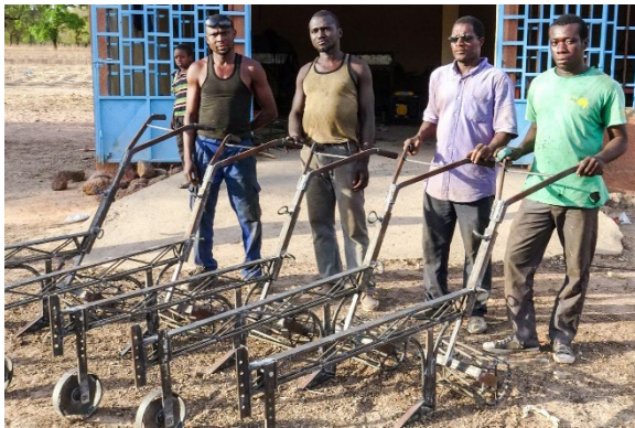
Local blacksmiths are now proficient in building and repairing in-line subsoilers for conservation cropping systems.
