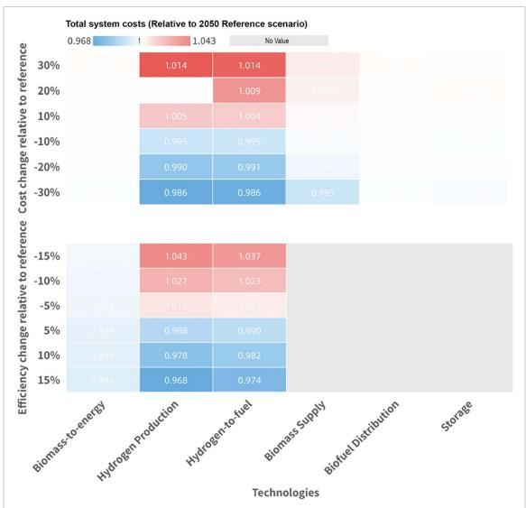
**Figure 8.** Sensitivity to technology costs and efficiency ('No Value', grey colour, represents that the uncertainty change is not applicable to the referred technologies; white colour (at the middle of colour scale) means the same system cost as in the 2050 Reference scenario, i.e. relative value = 1).
