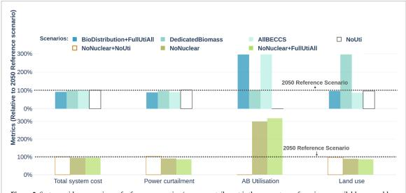
**Figure 5.** System-wide comparison of reference scenarios (power curtailment is the percentage of maximum available renewable electricity production from wind and solar photovoltaic technologies that is curtailed; AB utilisation is the percentage of the maximum available ancillary biomass potential which is used in a given scenario).
