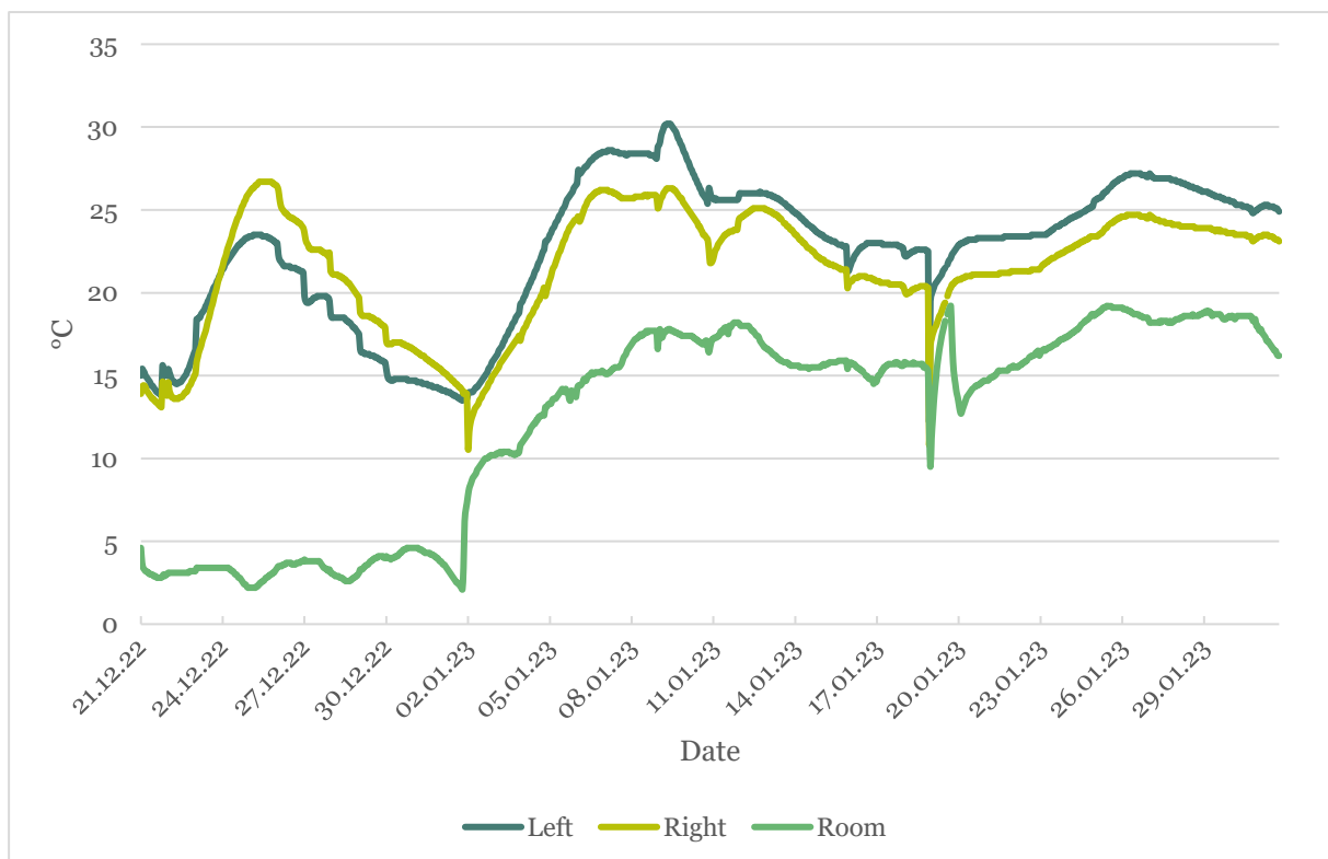
Figure 9 Temperatures recorded in compost tumbler from 21.12.2022-01.02.2023. The left chamber contained the original mix of Algae fiber and Leca®, the right chamber was given more Leca® on 02.01.2023. A heater was placed in the room on 02.01.2023, granulated sugar was added to both chambers on 09.01.2023, and the tumbler was moved to a smaller room on 19.01.2023.
