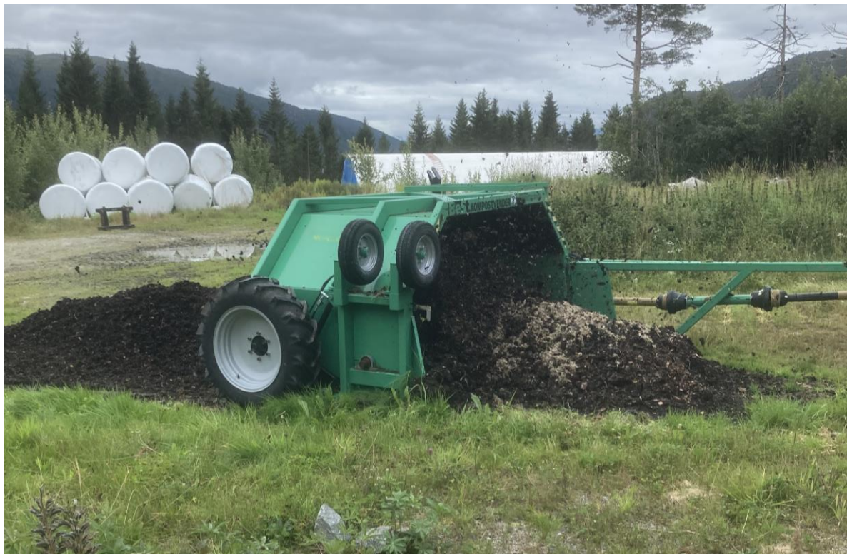
Image 12 Photo of the compost turner at Tingvoll Farm, taken on 26.08.2022. Visible on the right is a layer of acidified fish bone, on the left it is blended in. Photo: Anne-Kristin Løes.
