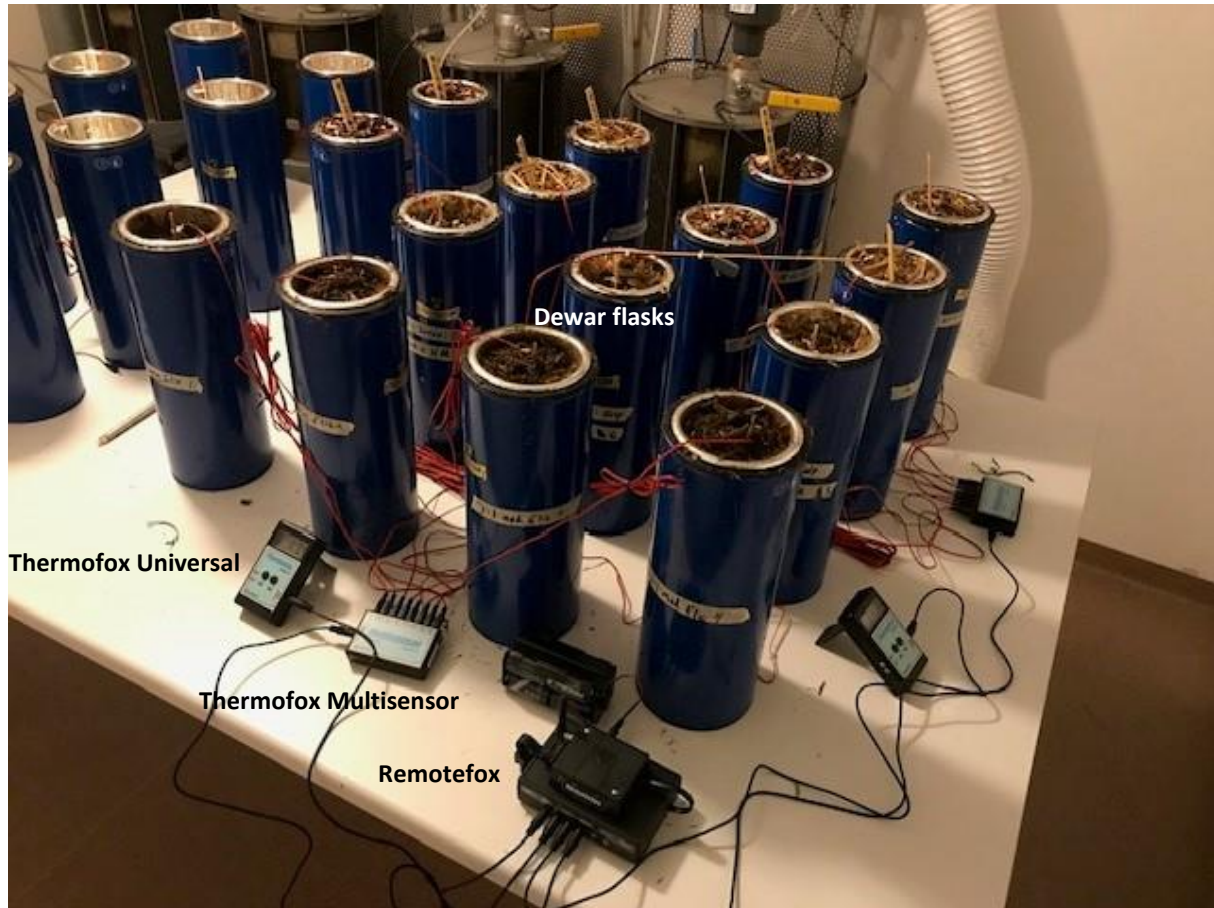
Image 9 Dewar flasks filled with feedstock. In front of and to the right of the flasks are two "Thermofox" and "Multisensor", and one "Remotefox" (bottom of photo). In later Dewar trials, the flasks were covered with a breathable cover to reduce heat and water vapor loss. Photo: Joshua Cabell.
