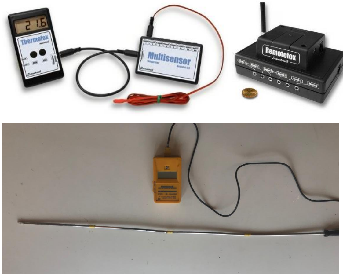
Image 13 Top left: Thermofox Universal; top middle: Thermofox Multisensor; top right: Remotefox; bottom: temperature probe from Sandberger. Photo: Scantronik (top), Joshua Cabell (bottom).
