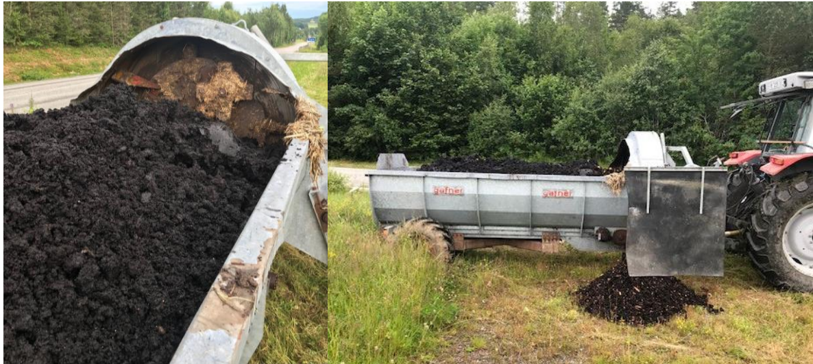
Image 11 Left: A view of the algae fiber (the other feedstocks are underneath) and the rotating knives of the Gafner; right: side view of the Gafner as it is depositing the mixed feedstocks. Photo: Joshua Cabell.
