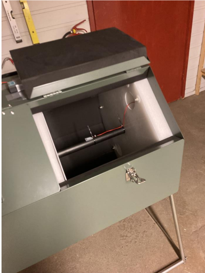
Image 10 Jordakompost 270 compost tumbler with one of the compartments open and a temperature sensor visible. The compartments were filled to just above the central axis halfway to the upper vent. Photo: Joshua Cabell
