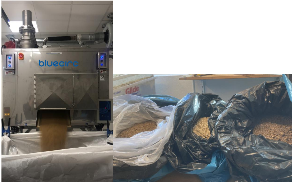
Image 8 Left side: drying, grinding, and sieving of fish spines (or whole fish in the case of “kleppafisk”) in a pilot project at Averøy, Norway in 2022 by BlueCirc AS. Right side: remains after sieving off the finest fractions for food and feed purpose. Photo: BlueCirc (l), Anne-Kristin Løes (r).
