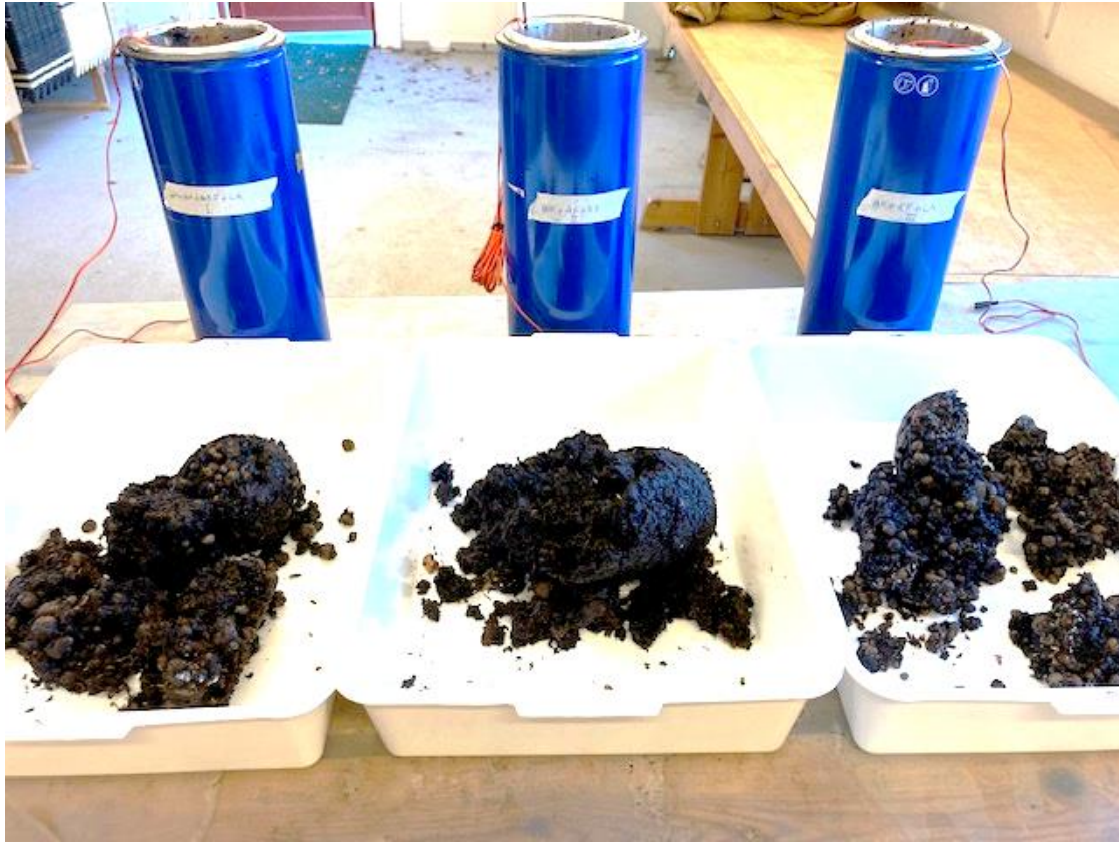
Image 18 Photo from the first Leca® trial taken on 14.11.2022. Horse manure + algae fiber + fish meal + Leca®; horse manure + algae fiber + fish meal; algae fiber + fish meal + Leca® (l-r). Photo: Joshua Cabell
