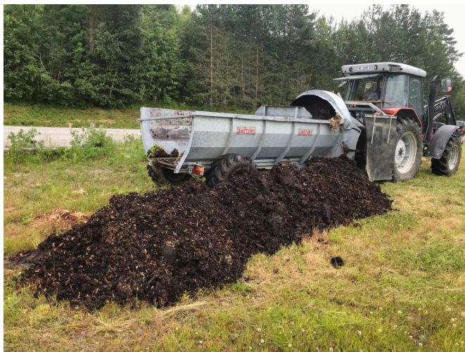
Image 14 The Gafner farmyard manure spreader with the windrow it just made. Photo: Joshua Cabell.
