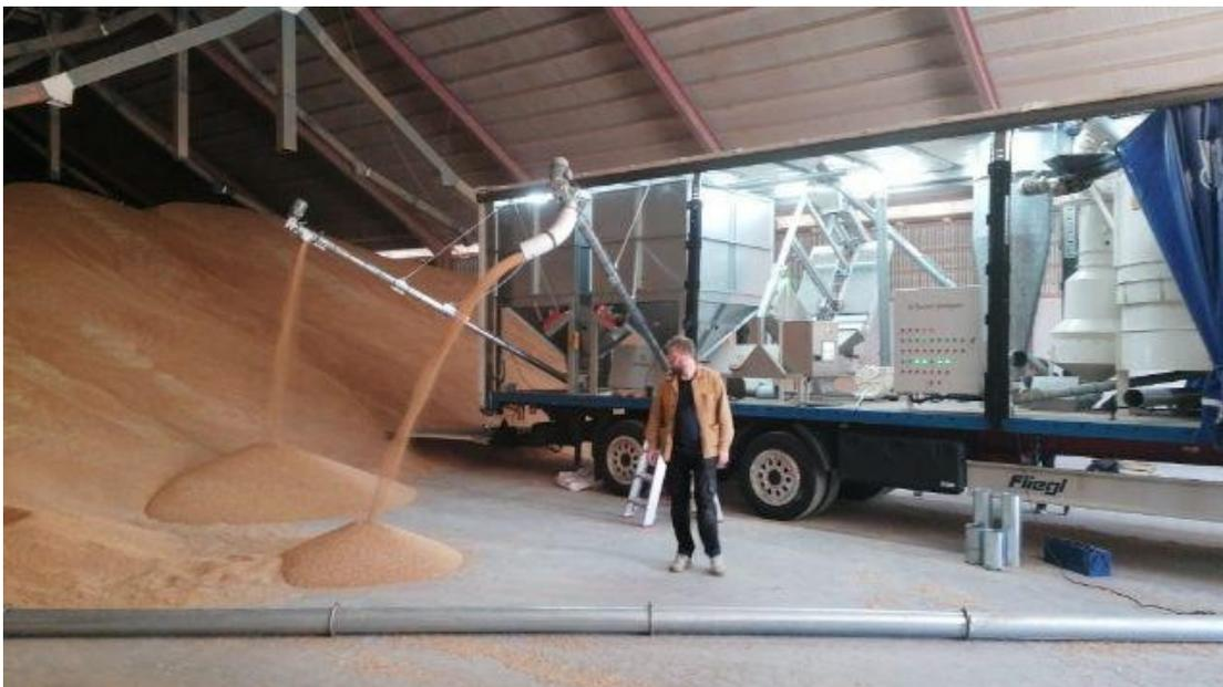
Figur 9: Quality improvement with [Gl.Buurholt's](#) novel mobile seed sorting equipment from [BoMill](#) .
