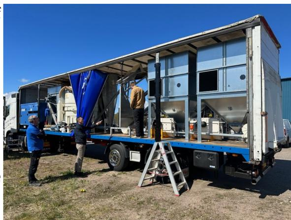
*Figur 3: The first inspection of the sensatinoal new equipment of a mobile factory with single seed sorting with NIT analysis with a capacity of 4 tonnes per hour*
