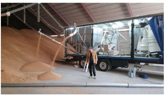
Figur 9: Quality improvement with <u>Gl.Buurholt's</u> novel mobile seed sorting equipment from <u>BoMill</u>.
