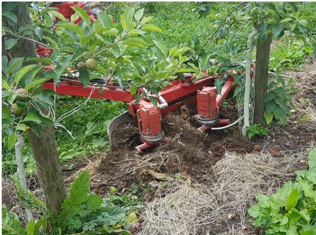
Picture 1. Gyroscopic crumbler by LADURNER in action, Photo: N. Oeser 2019.
