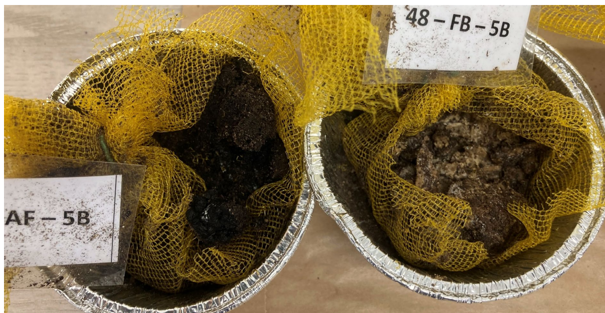
Picture 14. Algae fibre (AF) after three weeks of “storage” in soil; light brown spots had developed on the surface of the fibre. In acidified fishbones (FB), there was a lot of mould, and soil was attached to the bone surface. Photo by Anne-Kristin Løes, July 2, 2020.
