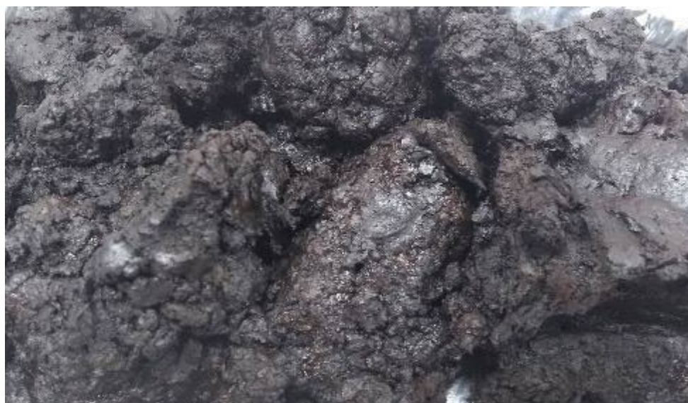
Picture 2. Algae fibre from Algea AS, Kristiansund. The product is a residue after chemical extraction of rockweed for liquid fertiliser and is a paste with about 25% dry matter. Photo by Ishita Ahuja.
