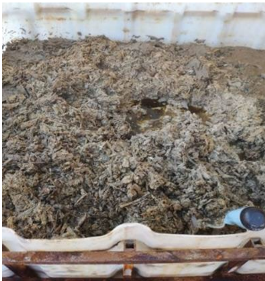
Picture 3. Sediment from hydrolysis of grinded residues of white fish (cod, saithe etc.) from Fjordlaks AS, ca. 50% dry matter. October 2018. Photo by Anne deBoer.
