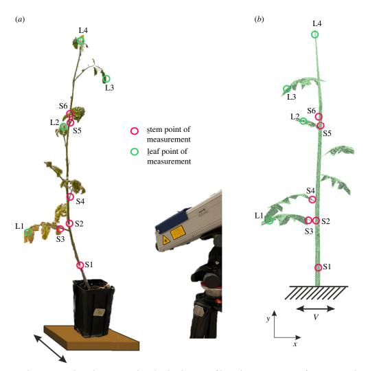
**Figure 1.** (a) Experimental setup to record signal propagation along the plant by means of laser vibrometer. Six points of measure were chosen along the stem (from S1 to S6, red circles) and four points on the leaves (L1–L4, green circles). (b) Three-dimensional FEM of a tomato plant, on which the same points were checked and compared with experiments.
