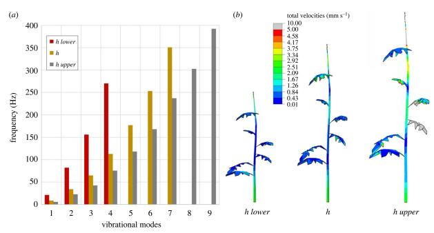
**Figure 7.** (a) Natural frequencies of S plant (height h) compared with the lower (h lower) and upper (h upper) case studies. Natural frequencies were extracted in the range of 0–400 Hz. (b) The comparison of the total velocity path through the plant by adopting one of the previous models.
