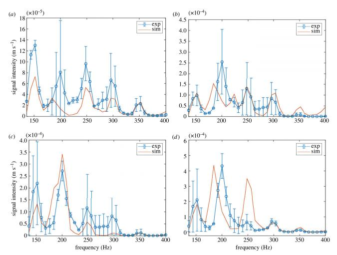
**Figure 4.** Comparison between numerical and experimental spectra of the recorded disruptive signal on the leaves of the plant (orange line and blue line with circles, respectively) for points L1 to L4 (a-d), respectively.
