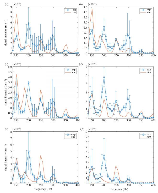
**Figure 3.** Comparison between numerical and experimental spectra of the recorded disruptive signal on the stems of the plant (orange line and blue line with circles, respectively) for points S1 to S6 (a-f), respectively.
