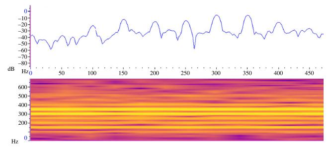
Figure 2. Background noise implemented with peaks of the amplitude corresponding to frequencies of 150, 200, 250, 300 and 350 Hz, with length of the signal of 1 s.
