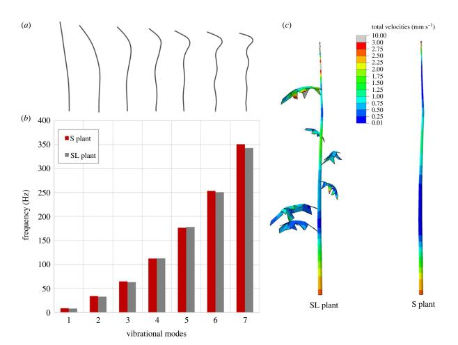
**Figure 6.** (a) Numerical vibrational modes of S plant, from mode 1 to 7. (b) Natural frequencies of S plant and comparison with SL plant (red and grey bars, respectively). (c) Vibrational velocity path through the plant by adopting a SL or a S plant model.
