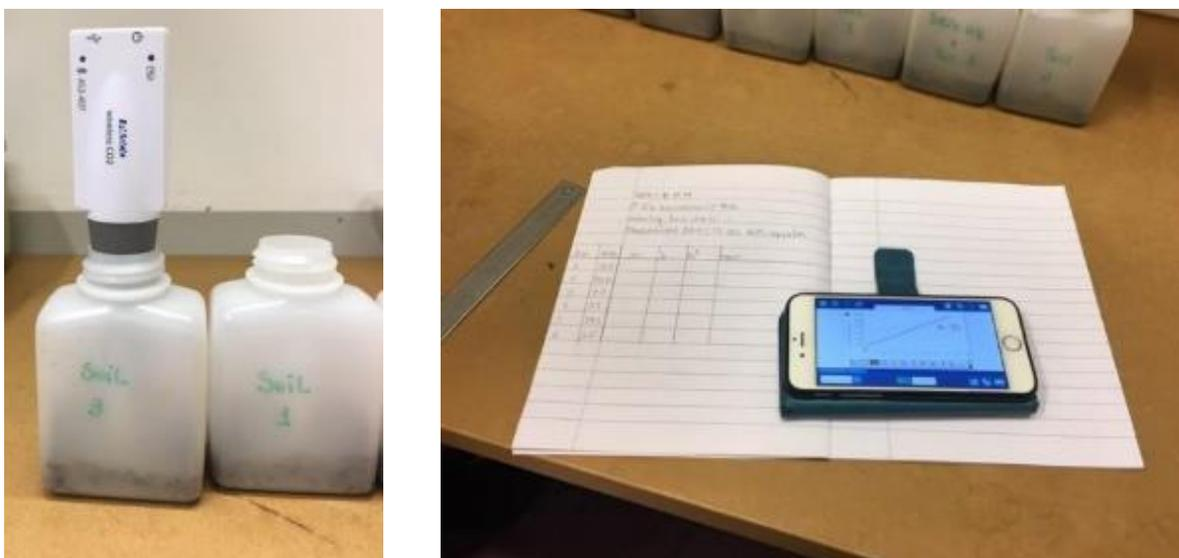
**Photo 8.** Left side: Pasco wireless CO<sub>2</sub> sensor during measuring the increase in CO<sub>2</sub> concentration inside a bottle with soil. Right side: Real-time measurement displayed on the mobile screen. Photos: Reidun Pommeresche, NORSØK.
