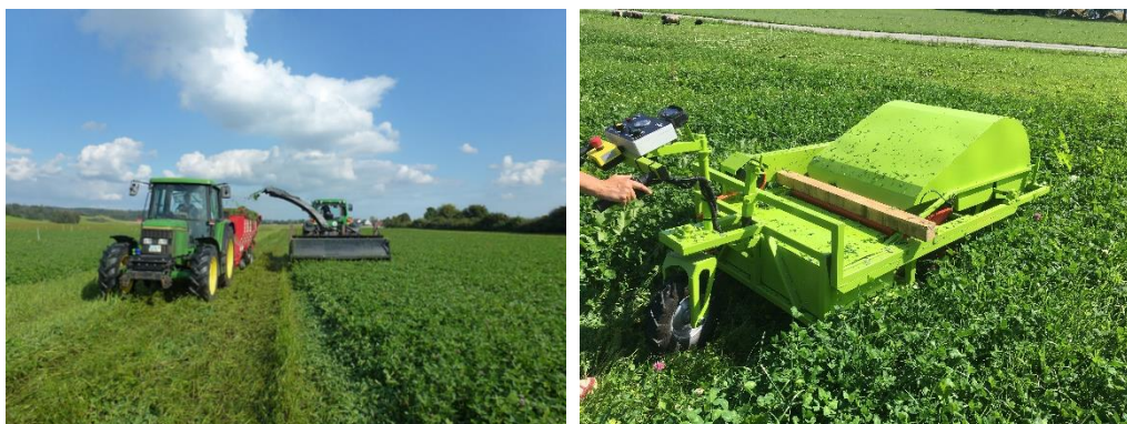
Leaf stripper prototype MFR1 (Trust'ing – Alf'ing) and the electric PremAlfa Mini developed by the same company in the ProRefine project for experimental use. Photos: Trust'ing – Alf'ing and Anne de Boer, NIBIO.
