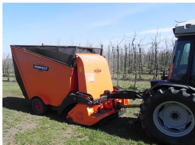
Picture 2: Leaf vacuum cleaner (Company PERFECT) used to remove fallen leaves from the tree strips in autumn (Photo: B. Benduhn, February 2014)
