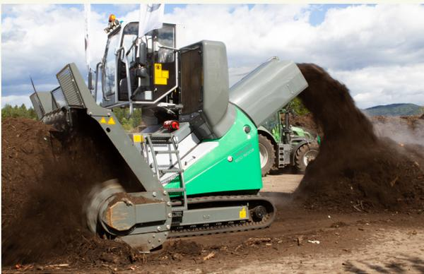
Fig. 2: Self-propelled, commercial compost turner.
