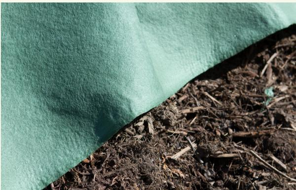
Fig. 3: Compost fleece prevents leaching and drying out.
