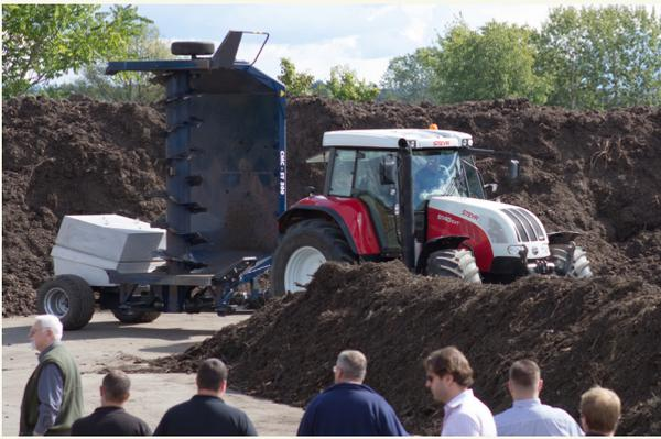
Fig. 1: tractor/PTO (power take-off) driven compost turner.
