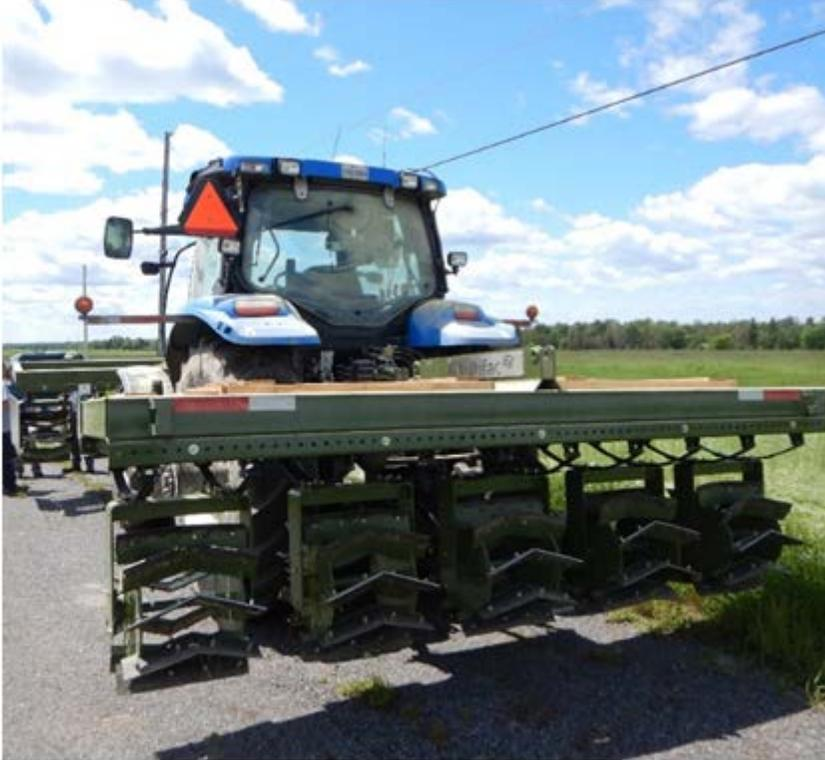
a. Modified roller crimper developed by a farmer in Eastern Canada
