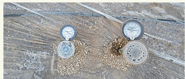
Fig. 1: Tensiometers to measure the soil humidity during solarisation. The left one is placed at 15 cm-depth, and the right one at 35 cm-depth.
