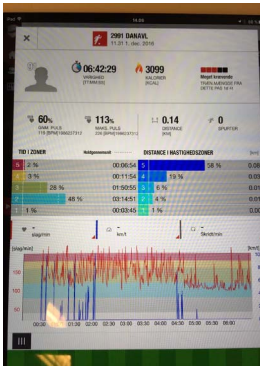
Figure 12. Illustration of method for estimation of sow locomotory activity with the Polar Team Pro equipment. The activity gauges were wrapped around the sows belly, and gel for ultrasound gestation scan was used to create permanent contact with the device. The system is initially developed for football players and provides heart rate, an activity map, and covered distance in different predefined velocity zones.
