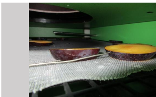
Picture 1 (left): Measurement of product temperature during drying of plums.
