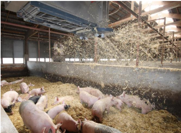
Figure 3: Silage and straw is distributed to the pigs in the pen. Photo: Ingela Löfquist.
