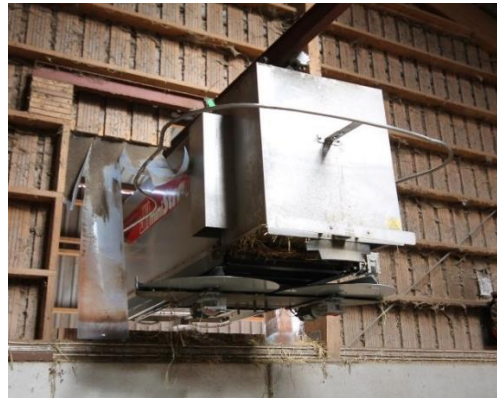
Figure 2: The automatic straw distributor entering the pig pen by a rail in the roof. Photo: Ingela Löfquist.
