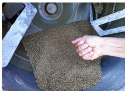
Figure: Vinegar treatment in a cement drum
