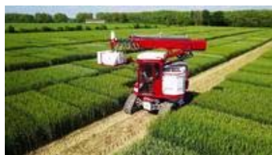
Phenomobile robot for in-field plant phenotyping, available at INRAE-Toulouse
