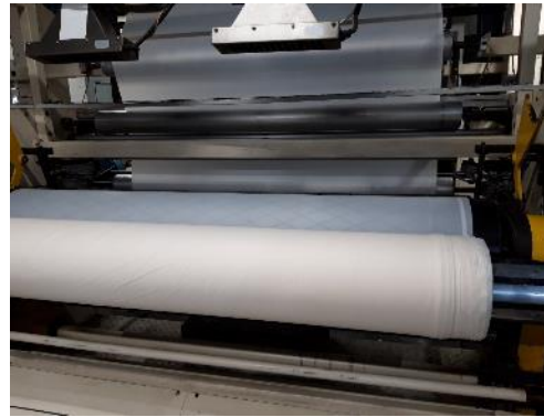
Melting → blowing → cooling → winding on the spool
