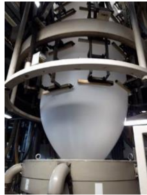
Melting → blowing → cooling → winding on the spool
