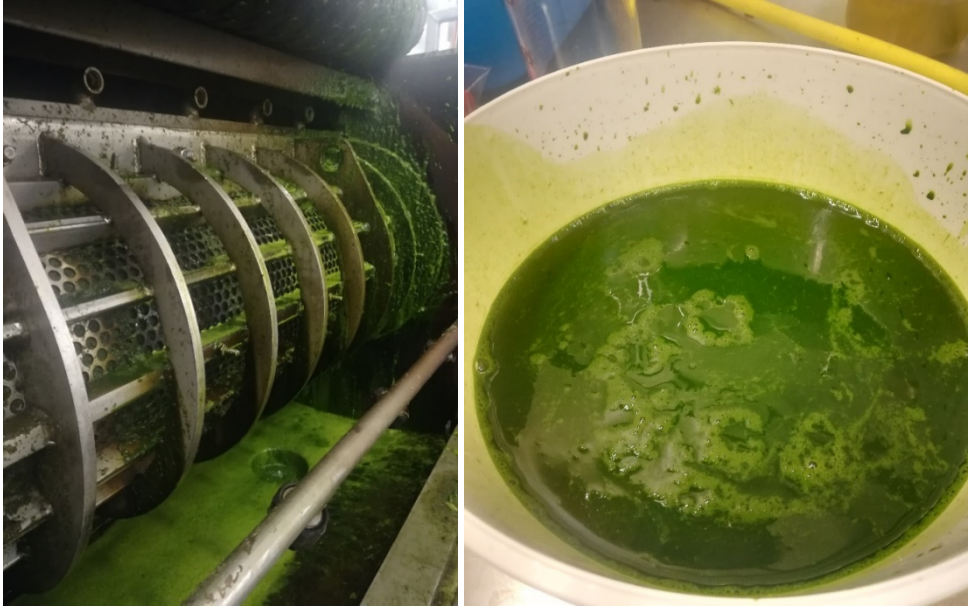
Juice squeezed out from fresh alfalfa in a screw press at the pilot plant.
