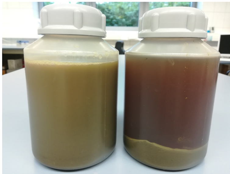
Separation of proteins after centrifugation of the juice treated with lactic acid bacteria.
