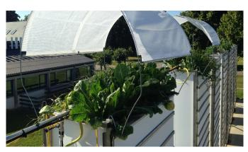
We grew chicory (Cichorium intybus L.) in these 4 m tall soil filled rhizotrons. TDR sensors logged the volumetric water content continuously. Late season, two treatments were established. "Wet", where water was supplied regularly to avoid water limitations and "Dry" where no water was supplied.
