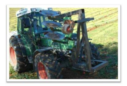
Figure 2 5 Disc-harrow machine in transport position, performed at the farm for mobilization along the line by the sandwich method
