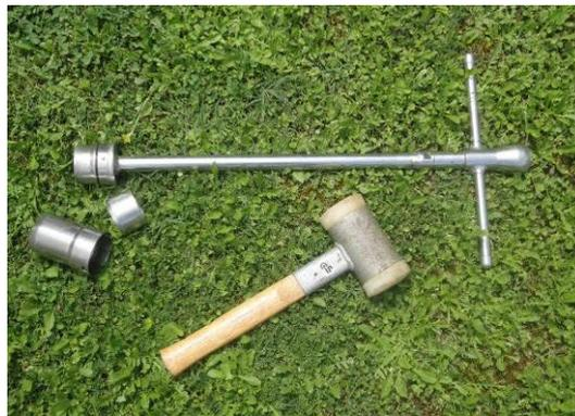
Figure 2. Hammer-driven double-cylinder sampler
