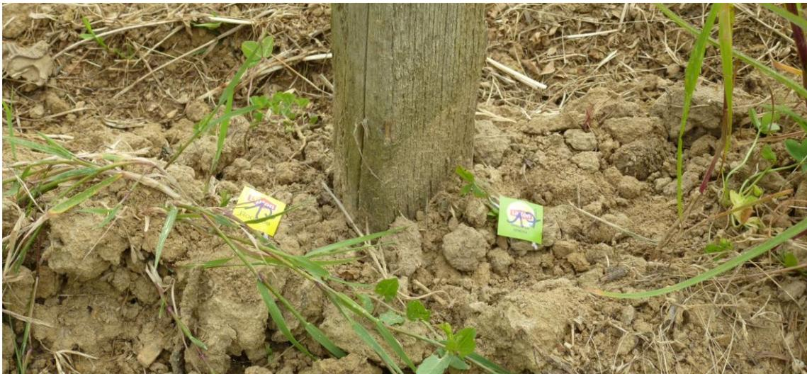
Figure 8. Two types of teabags buried with visible labels
