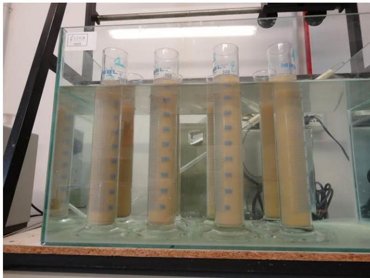
Figure 5. Soil particle-size analysis by the pipette method.
