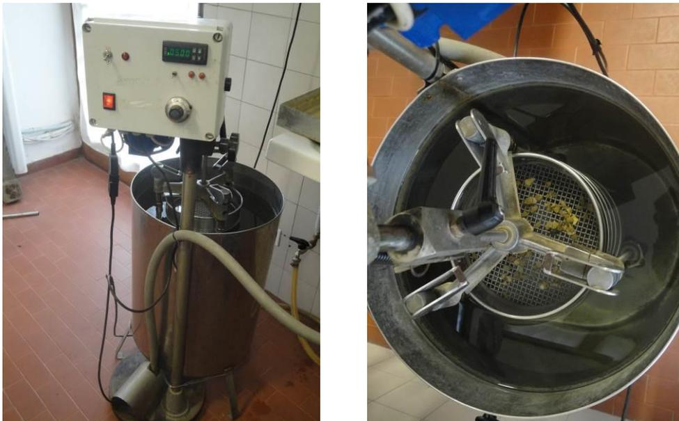
Figure 7. The electronic-controlled machine for aggregate stability analysis by wet sieving.
