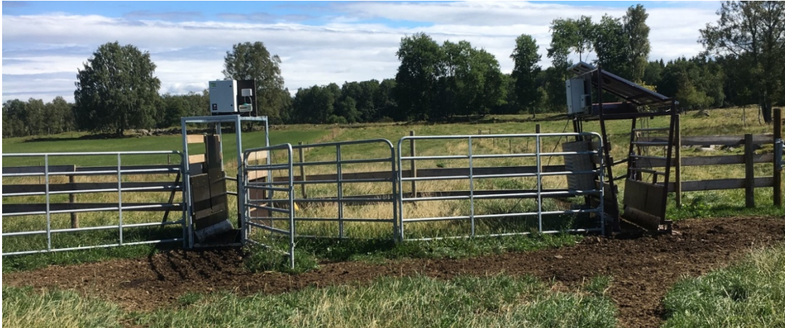
Figure 3. Shows a picture of the two automatic weighing stations. The scale to the right was operated on solar cells and the scale to the left was operated on line current (Photo: Lisa Johansson).
