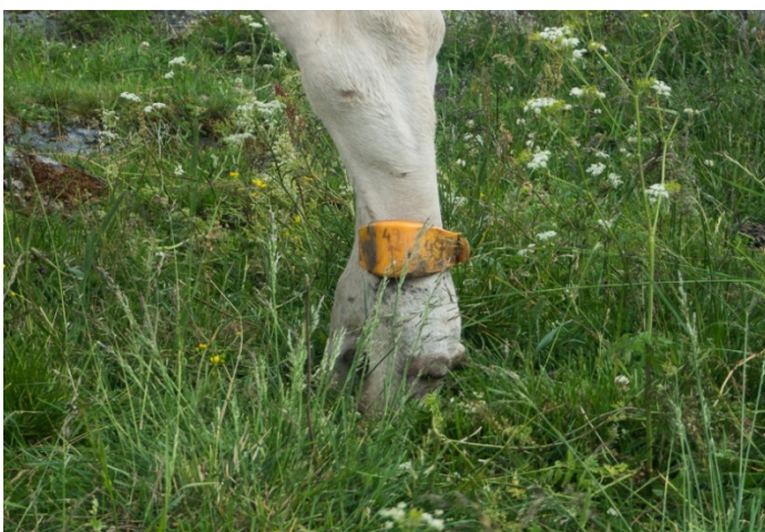
Figure 4. A picture of an IceTag, which is a device that record the activity level (Photo: Katarina Arvidsson Segerkvist).
