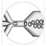
Sample is partitioned into many thousands of nanoliter droplets
