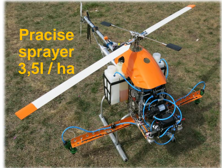
flight time– 2 h, lifting capacity – 10 kg
