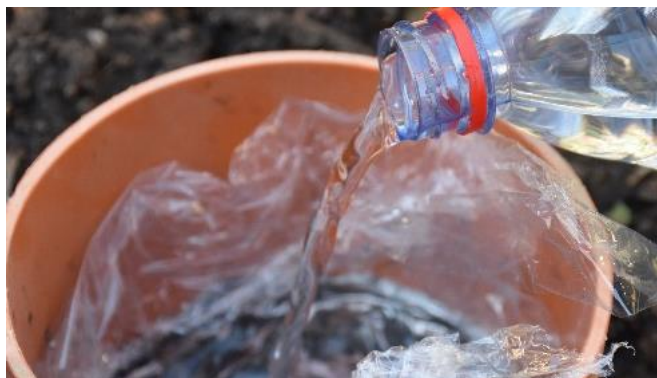
Image 3: The measured amount of water is poured into the ring on the foil. (Image: Boris Liebl, FiBL).
