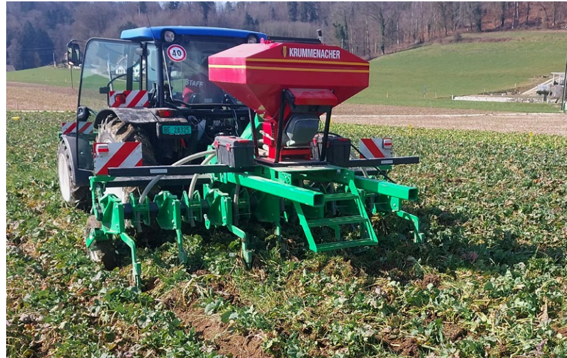
With the dam forming plough, primary tillage, sowing and weed control can be carried out with a single pass in crop cultivation.
