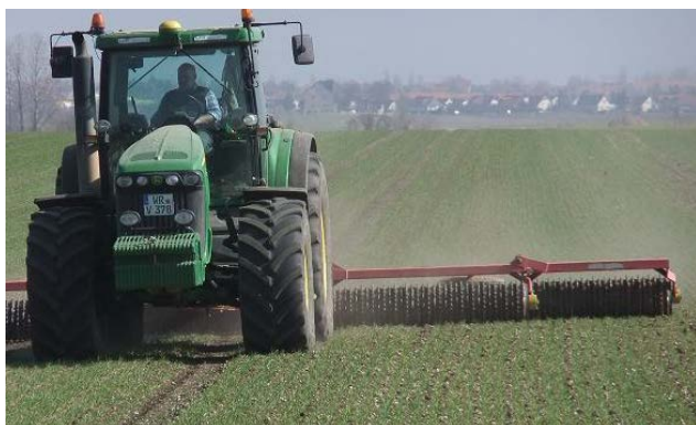
Figure 1: Rolling winter wheat (with corrugated roller in the photo) is supporting seed-soil contact and stimulates tillering. (Photos: www.gut-derenburg.de )
